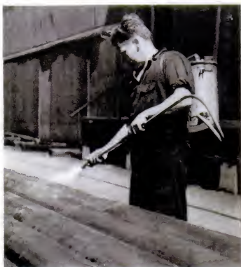
Applying the liquid coating to metal with a spray
